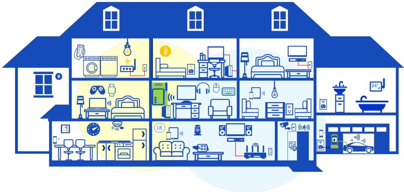
Figure 13 – Example 2 “Improved connectivity to RG” utilizing Wi-Fi Repeater/Extender
