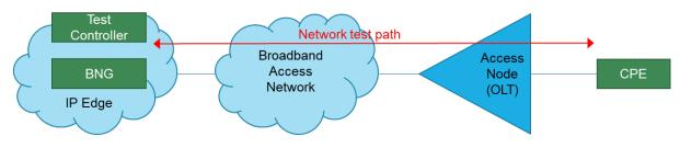
Figure 3: IP Edge to CPE measurement of Maximum IP Capacity
