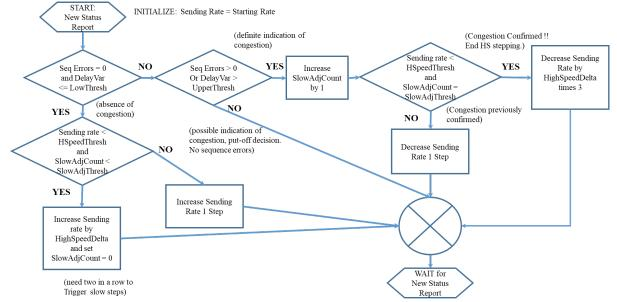
Figure 4: Flowchart for Offered Load adjustment as part of the "B" Search Algorithm
