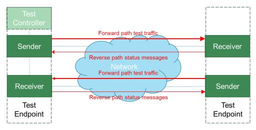
Figure 2: Maximum IP Capacity measurement reference architecture
