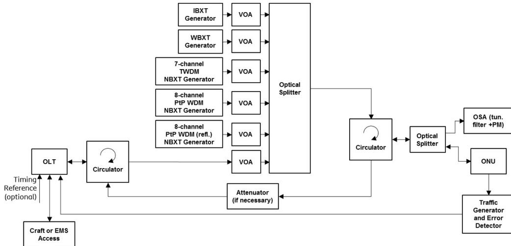
**Figure 12.1 – Simplified Test Setup for ONU Receive Sensitivity**
