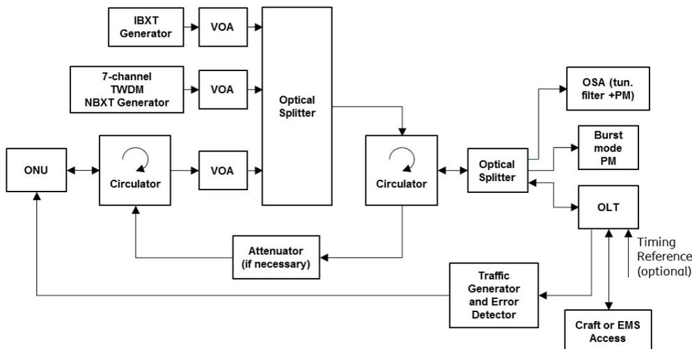
**Figure 16– Test Setup for OLT Receive Sensitivity**
