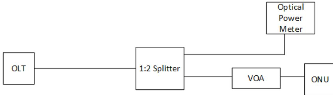
**Figure 15 – Test Setup for OLT Transmit Power**
