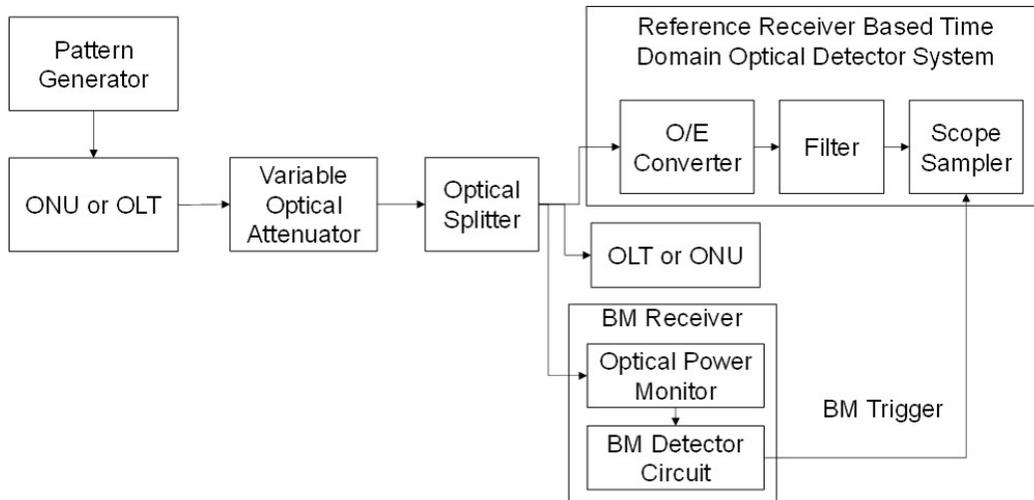
Figure 2 - Optical eye pattern, waveform, and extinction ratio measurement configuration
