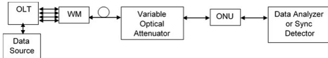
**Figure 8 – Test Setup for ONU Receiver Tuning Time**
