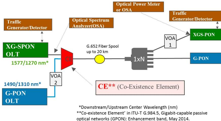
Figure 17 – Test Setup for XGS-PON ONU Coexistence with GPON
