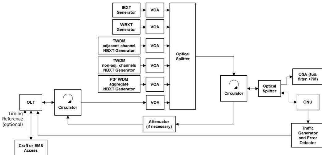
**Figure 12.2– Simplified Test Setup for ONU Receive Sensitivity**
