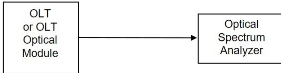
**Figure 14 – Test Setup for OOC and OOB PSD****Discussion**
