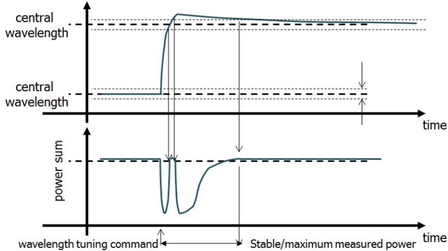
**Figure 7 - Optical power vs. time from summation of waveform monitors**
