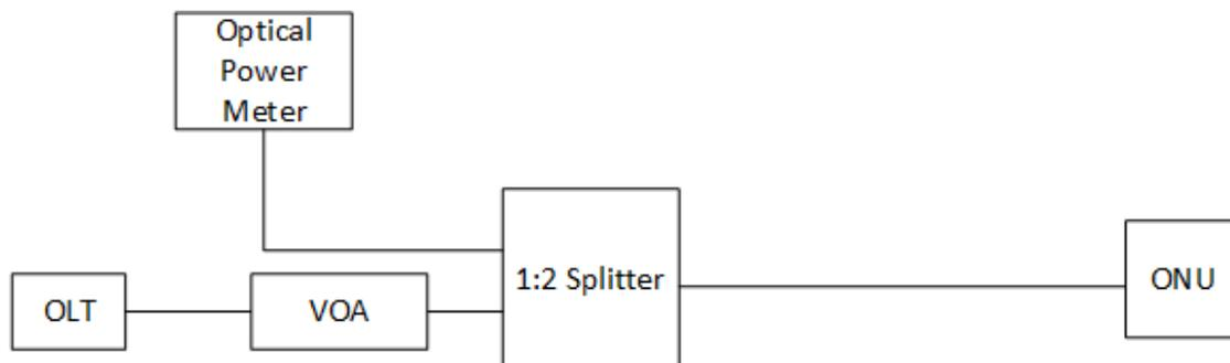
**Figure 10 – Test Setup for ONU Transmit Power**
