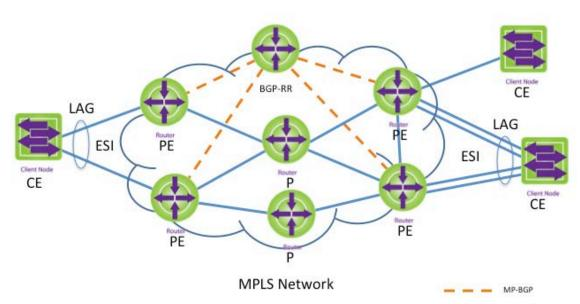
Figure 3 EVPN Architecture for Ethernet services using BGP MPLS
