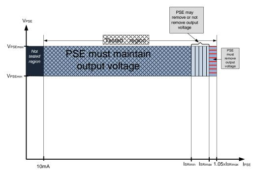
Figure 7-1 – Allowed tested region for  $V_{PSE}\mbox{-}I_{PSE}$  diagram
