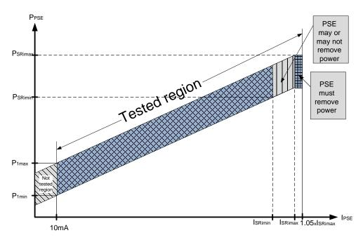
Figure 7-2 – Allowed tested region for  $P_{PSE}$ -I<sub>PSE</sub> diagram
