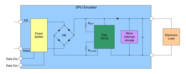
Figure 7-3 - DPU Emulator for PSE standalone testing (example)
