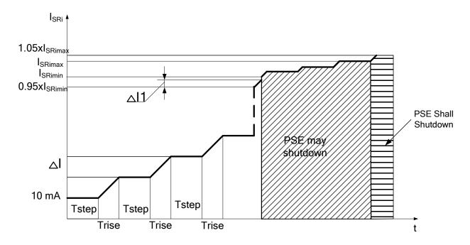
Figure 6-7 – Electronic Load (I<sub>SRi</sub>) increments
