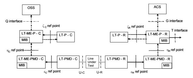
Figure 1: Functional reference model of DSL line test
