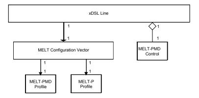
Figure 5: MELT configuration model
