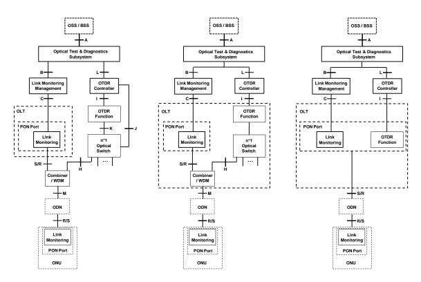
Figure 2 – Reference architectures for external, chassis-based, and dedicated OTDR (left to right).
