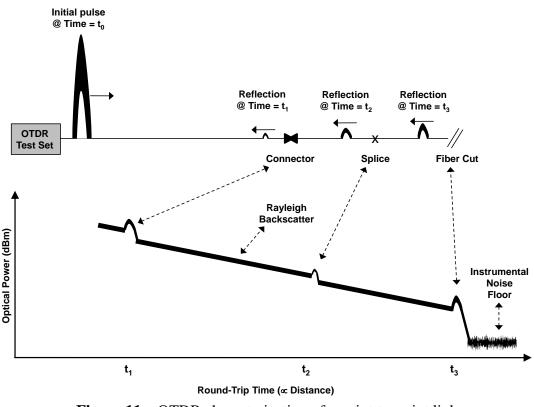
Figure 11 – OTDR characterization of a point-to-point link.
