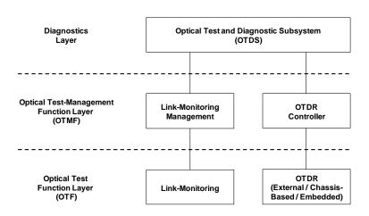
**Figure 1** – Logical functional blocks of an OLM system.
