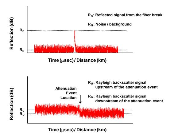
Figure 14 – Detection criteria for fiber faults.
