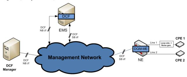
Figure 2 – Test Configuration for functional tests - Distributed DCF external, connected to a single NE
