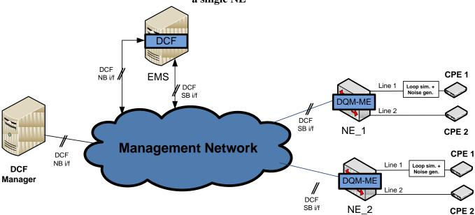
Figure 3 – Test Configuration for functional tests - Distributed DCF external, connected to multiple NEs
