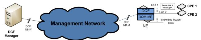
Figure 4 – Test Configuration for performance tests - Distributed DCF in the NE
