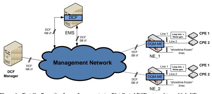
Figure 6 – Test Configuration for performance tests - Distributed DCF external to multiple NEs
