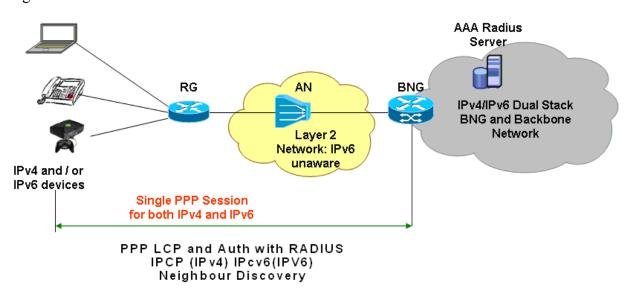
Figure 4: Example IPv6 Connectivity with PPP Session Initiated by a Host behind the RG
