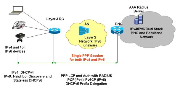
Figure 3: Example IPv6 Connectivity with PPP Session Initiated by the RG
