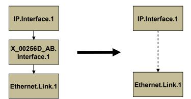
Figure 7 – Ignoring a Vendor-specific Interface Object in the Stack
