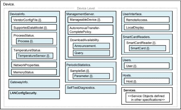
Figure 2 – Device: 2 Data Model Structure – Device Level
