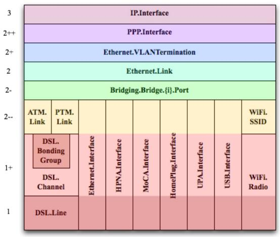
Figure 5 – OSI Layers and Interface Objects<sup>1 2</sup>
