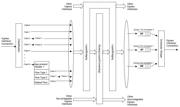
Figure 10 – Queuing Model of a Device
