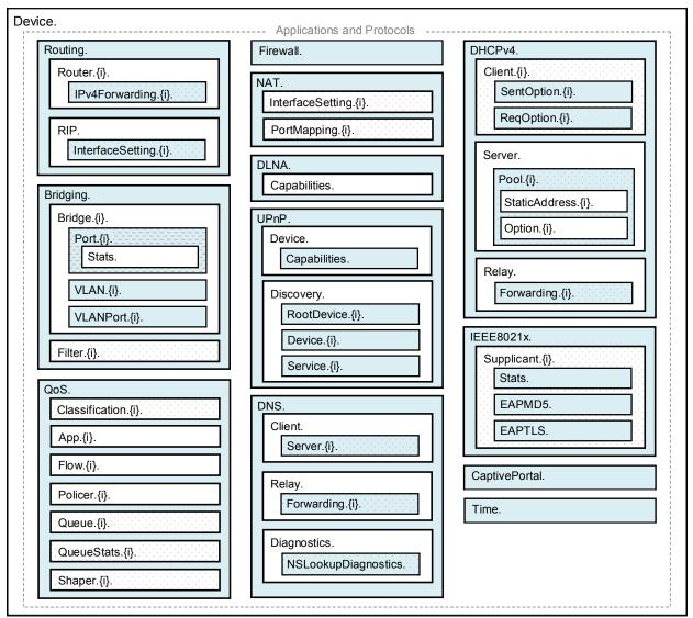
Figure 4 – Device:2 Data Model Structure – Applications and Protocols
