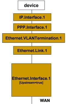
**Figure 16 – VLAN Termination model**
