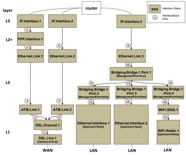
Figure 9 – Simple Router Example (Interfaces Visualized)
