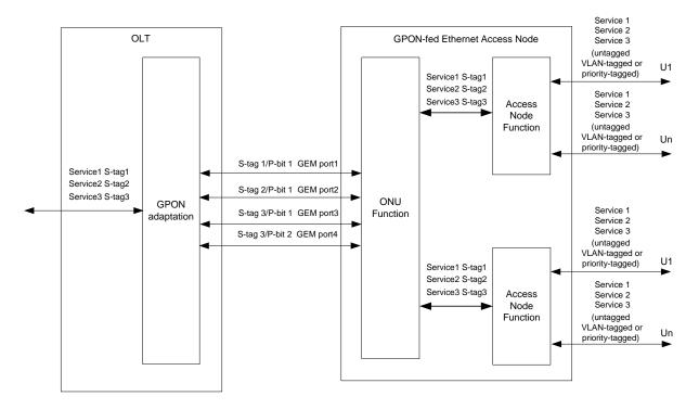
**Figure 5 – Frame mapping for GPON-fed Ethernet access node**
