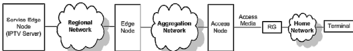
Figure 4 – IPTV End-to-End Network Components
