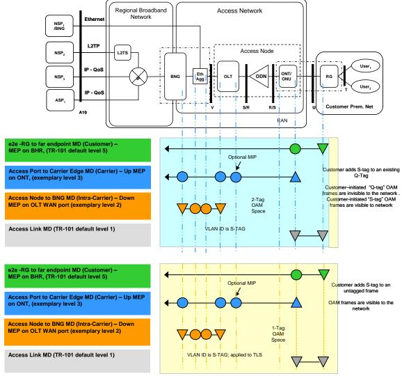
Figure 23 – Ethernet CFM for Customer-S-tagged TLS VLANs
