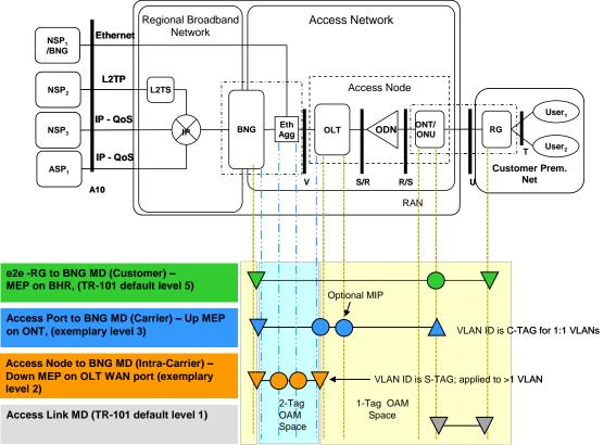
Figure 19 shows where the MEPs and MIPs are placed for 1:1 VLANs.
