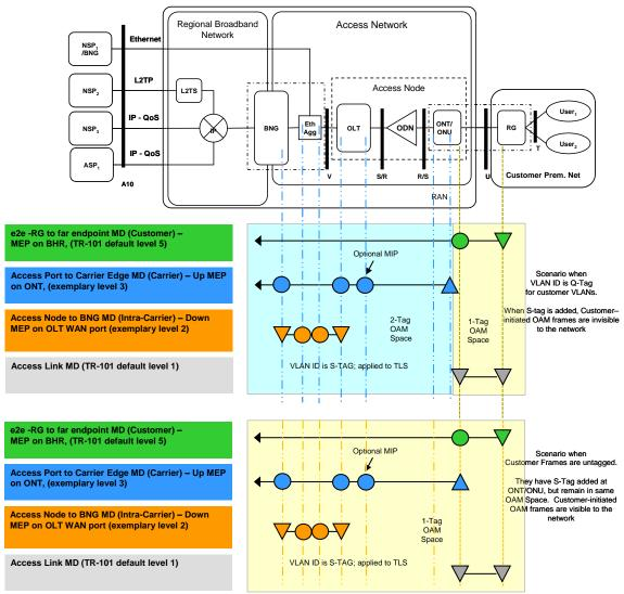
Figure 22 – Ethernet CFM for Carrier-S-tagged TLS VLANs
