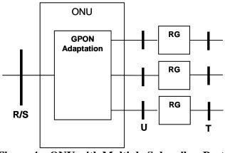
**Figure 4 – ONU with Multiple Subscriber Ports**
