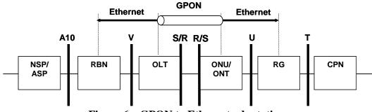
Figure 6 – GPON to Ethernet adaptation
