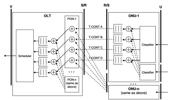
Figure 16 – Upstream Queuing and Scheduling Model Example
