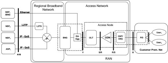
Figure 1 – Network architecture for Ethernet-based GPON aggregation
