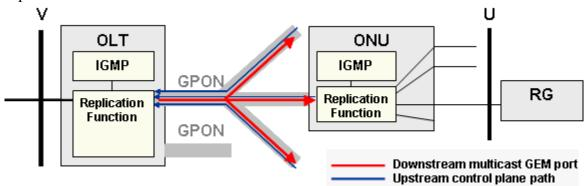
Figure 18 – GPON Multicast GEM ports
