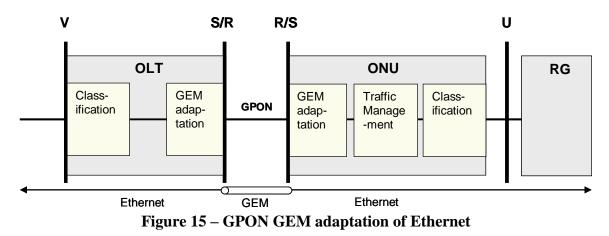
The general requirement for GEM is to provide QoS mechanisms that can support the Ethernet QoS requirements of TR-101. By doing this, the set of access node QoS requirements defined in Section 3.3/TR-101i2, still apply to the Ethernet domain of the GPON distributed access node.
