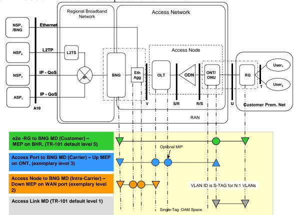
Figure 21 where the MEPs and MIPs are placed for N:1 VLANs.
