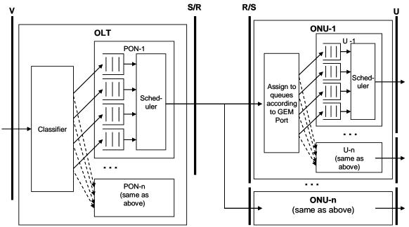
**Figure 17 – Downstream Queuing and Scheduling Model Example**
