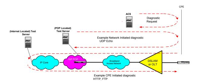
Figure 1 Performance testing components
