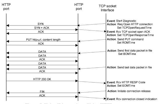
Figure 7 UploadDiagnostics utilizing HTTP transport
