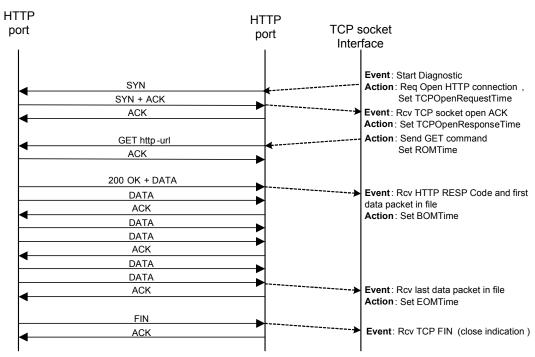
Figure 6 DownloadDiagnostics utilizing HTTP transport
