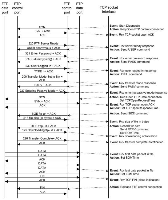
Figure 4 DownloadDiagnostics using FTP transport
