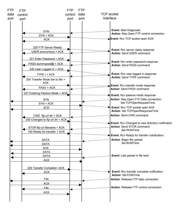
Figure 5 UploadDiagnostics utilizing FTP transport
