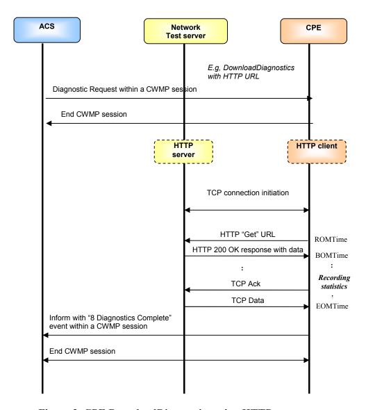
Figure 2 CPE DownloadDiagnostics using HTTP transport.
