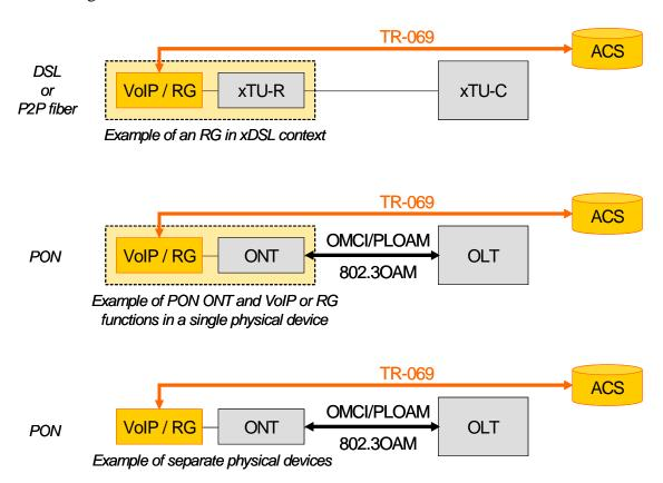
Figure 3: Example of TR-069 versus OMCI configuration and management.
