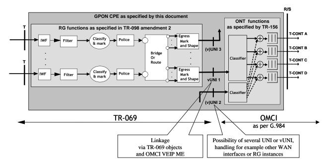
Figure 5: Representation of the upstream traffic; OMCI and TR-069 management of a multi-port single-subscriber GPON CPE
