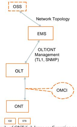
Figure 1: Example of ONT link layer configuration and management.
