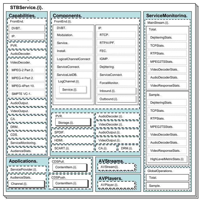
Figure 2– TR-135 – STBService object structure
