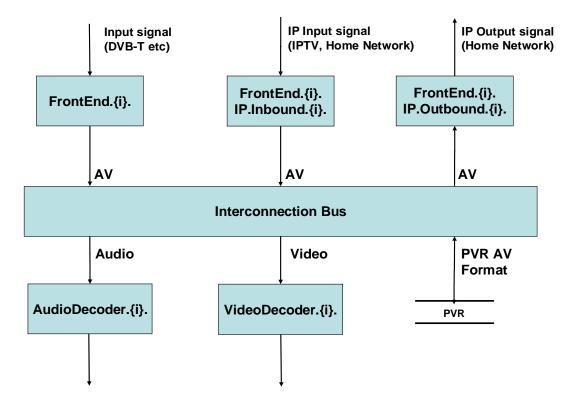
Figure 3- Logical AV Streaming Model
