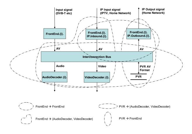
Figure 4 – Logical AV Streaming Model with Example Streams
