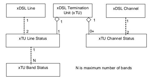
Figure 3/TR-129 - Managed object model: xDSL status monitoring
