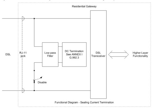
Figure 18 – Sealing current reference design
