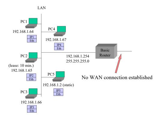
Figure 6 – Example: No WAN Connection Configuration
