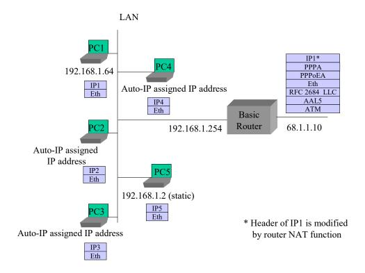
Figure 13 – Example: Single PC Mode of Operation
