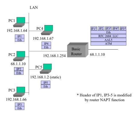
Figure 10 – Example: Router in 2684 Bridged Mode with DHCP Server On
