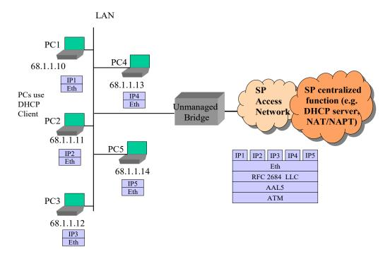
Figure 17 – Example: Unmanaged Bridge Configuration
