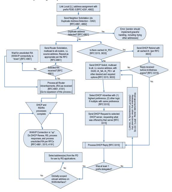
Figure 3 – WAN IPv6 automated connection flow
