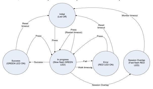
Figure 1 – WPS pushbutton method state machine
