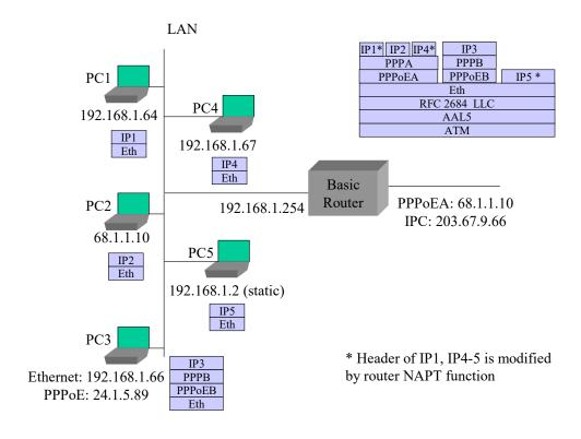
Figure 15 – Example: Router sets up Second IP Connection
