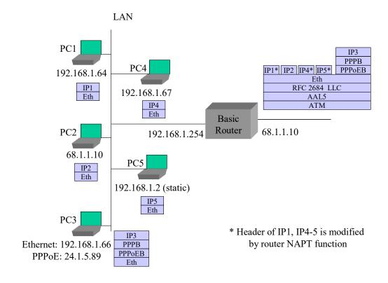
Figure 14 – Example: Router in Routed 2684 Mode
