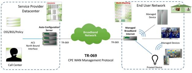
Figure 1 – CWMP Positioning in the End-to-End Architecture
