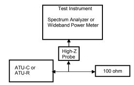
Figure 4-3 - Test Configuration for PSD Measurement Tests
