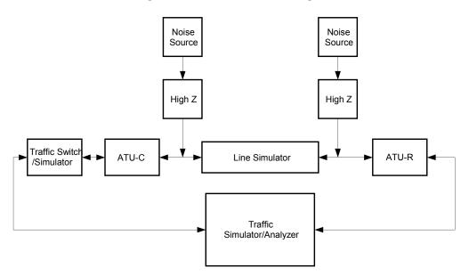
Figure 4-2 Test Setup for Configurations Using Data Layer
