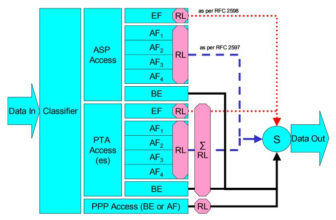
Figure 1 - Queuing and Scheduling Example for DSL Router
