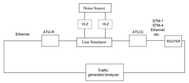
Figure 4: Test set-up for Ethernet modems
