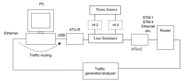
Figure 5: Test set-up for USB modems
