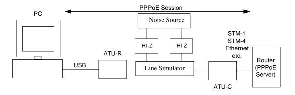
Figure 13: Test setup for PPPoE testing with USB modems
