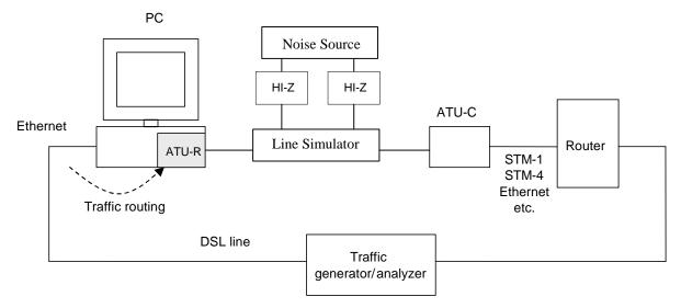
Figure 6: Test set-up for PCI (internal) modems
