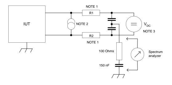
NOTE 1: These resistors have to be matched: R1=R2=R<sub>T</sub>/2 and R1/R2=1 +/-0.1%. NOTE 2: For LTU test only if remote power feeding is supplied. NOTE 3: For NTU test only if remote power feeding is required DC blocking capacitors=C<sub>B</sub>.
