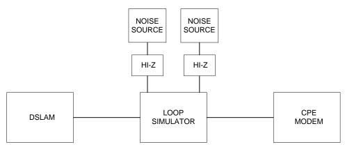
Figure 1: Test setup for loop tests for ADSL external modems
