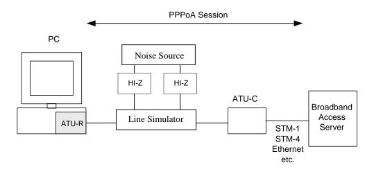
Figure 17: Test setup for PPPoA testing with PCI modems
