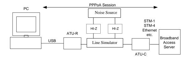
Figure 16: Test setup for PPPoA testing with USB modems
