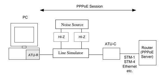
Figure 14: Test setup for PPPoE testing with PCI modems
