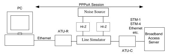
Figure 15: Test setup for PPPoA testing with Ethernet modems
