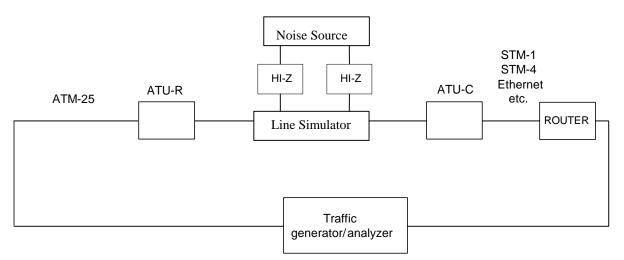
Figure 3: Test set-up for ATM-25 modems
