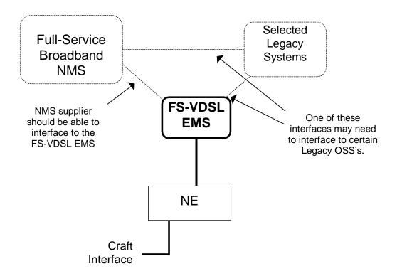
Figure 2 Example of an FS-VDSL Network Management Architecture
