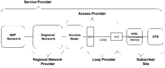
Figure 1 – Example DSL Network Components
