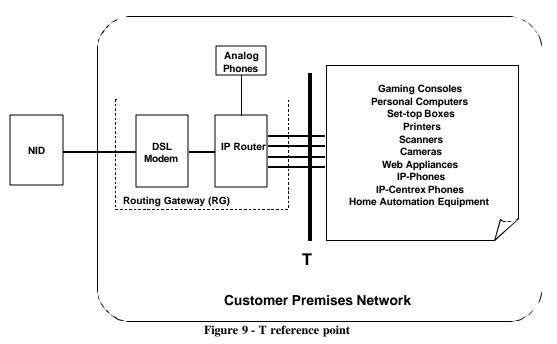
Figure 9 also shows a link with one or more analog phones. This would be the case for an Integrated Access Device (IAD) offering derived voice. There are two possibilities to offer packetized voice to the access network:
