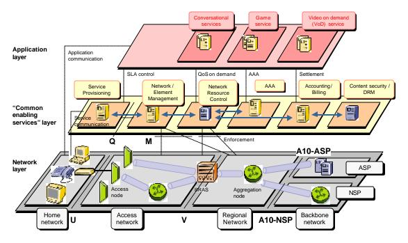
Figure 4 - Three-layer logical/functional architecture for support of advanced services
