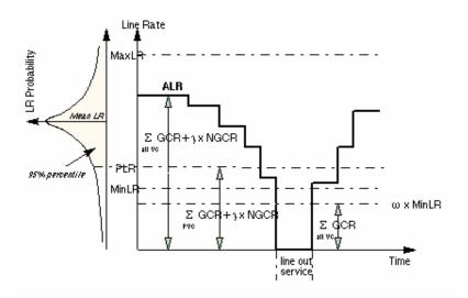
Figure 3 - Line rates, CAC and probability in rate adaptive DSL networks
