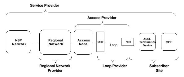
Figure 10 - DSL Network Components (Voice and application components not shown for clarity)
