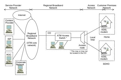
Figure 2. Example of an end-to-end DSL-based Broadband Network Architecture
