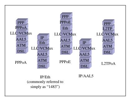
Figure 3: Protocol Stacks at the "U" Interface
