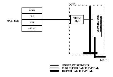
Figure 9. Integrated POTS and ADSL Line Card
