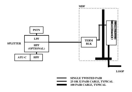
Figure 8. POTS Splitter Located Near PSTN Switch
