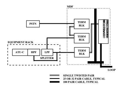
Figure 4. POTS Splitter Located near ATU-C
