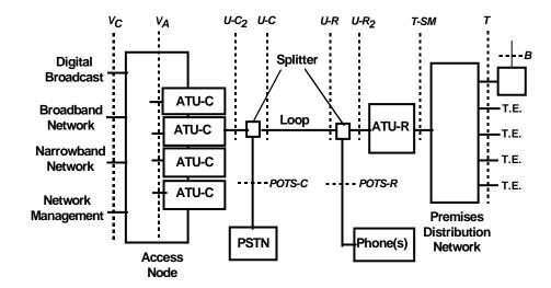
Figure 10. (below) presents The Broadband Forum System Reference Model for ADSL network systems.
