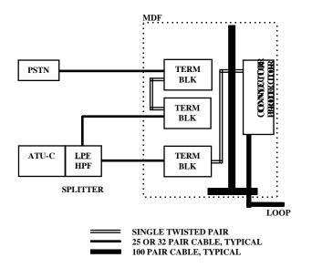
Figure 3. POTS Splitter Located with ATU-C
