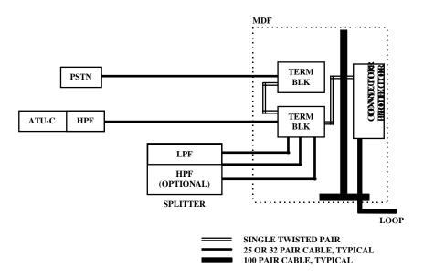
Figure 6. POTS Splitter Located Near MDF
