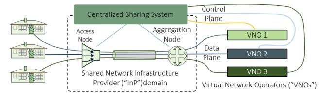
Figure 1. Network sharing, showing network slices in different colors.
