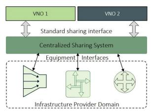
Figure 2. Management System based Sharing: management plane
