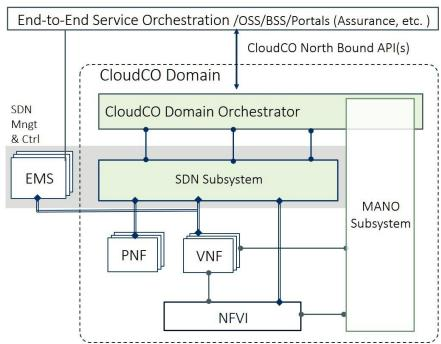
A CloudCO '*Domain*' is an ensemble of network, compute, storage, and application components that work together to deliver networking and customer services, located in one or more network sites, are orchestrated by a single CloudCO Domain Orchestrator and share a common, uniquely addressable CloudCO northbound interface.
