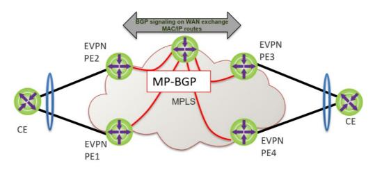
Figure 1: EVPN for next-generation Ethernet services on MPLS.
