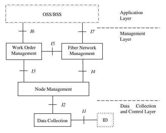
Figure 2 Architecture of fiber infrastructure management system
