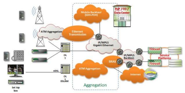
Figure 2 –Network Architecture of SP2
