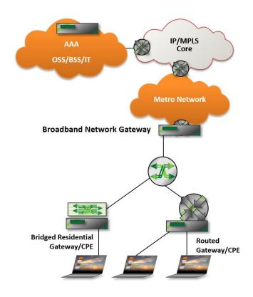
Figure 1 –Network Architecture of SP1
