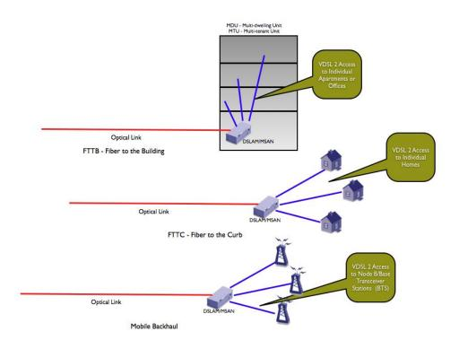
Figure 9 - Schematic of Deployment Architectures
