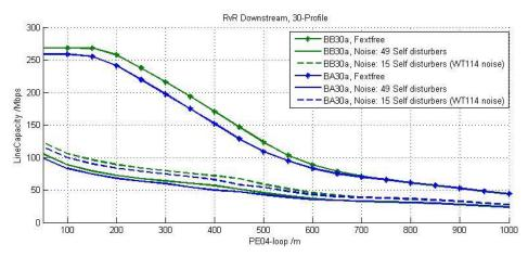
Figure 8 - VDSL2 Annex B Profile 30a downstream loop reach and rate
