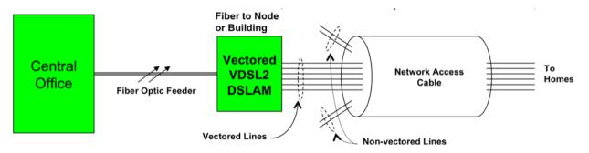
Figure 2 - Reference Fiber Fed DSL Network Access Architecture
