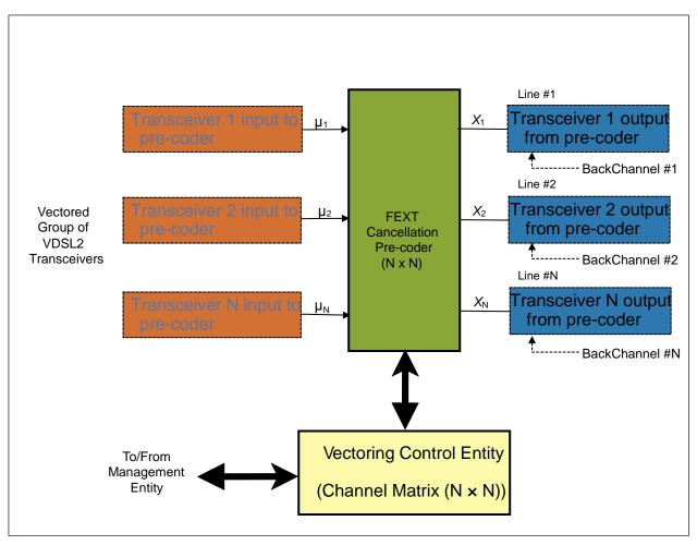
Figure 4 - Downstream FEXT Cancellation Pre-coding in DSLAM
