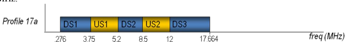
Figure 5 - Example band plans for profile 17a
