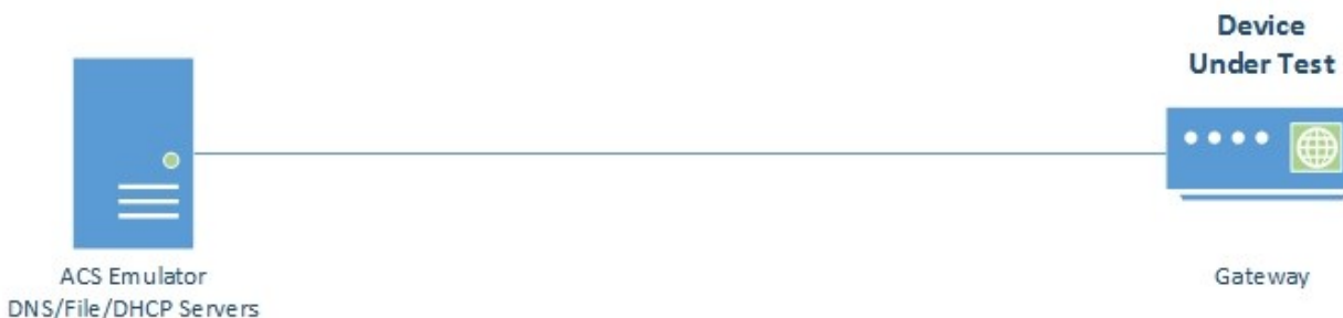
Figure 1: RG Test Setup via Ethernet
