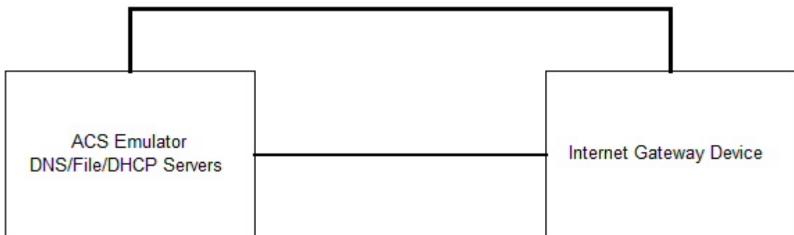
Figure 1: RG Test setup via Ethernet
