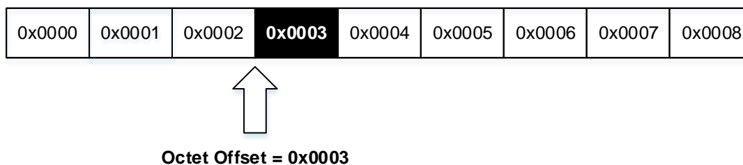
Figure 3.2: Writing Data to an Offset Position
