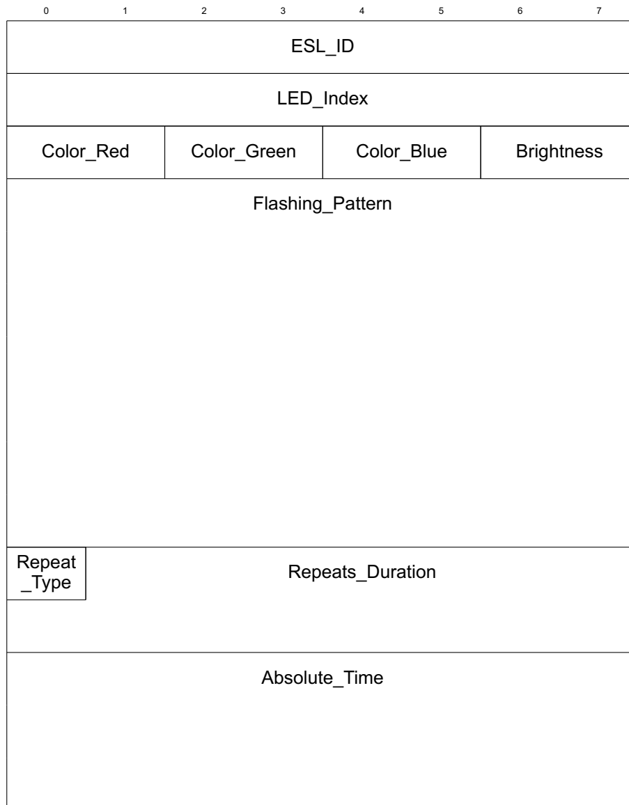
Figure 3.13: LED Timed Control command parameters
