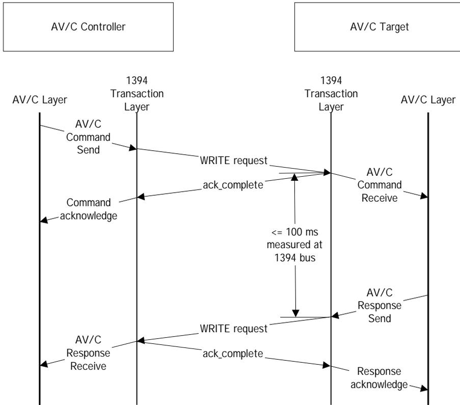
Figure 8.4 – Anatomy of an AV/C transaction with 1394 unified transactions
