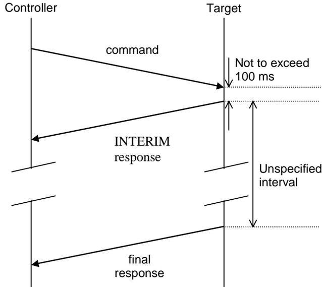
**Figure 8.2 – AV/C deferred transaction**
