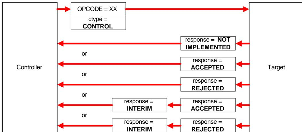
Figure 9.1 – Command and responses for CONTROL commands
