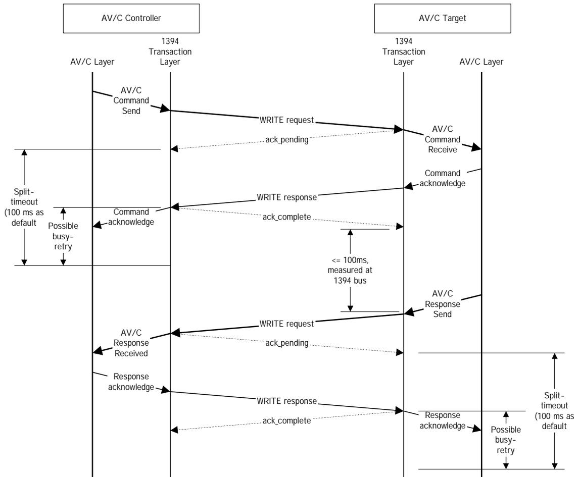
Figure 8.3 – Anatomy of an AV/C transaction with 1394 split transactions
