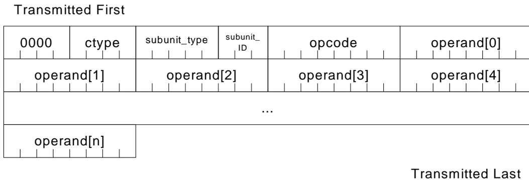
**Figure 7.1 – AV/C command frame**
