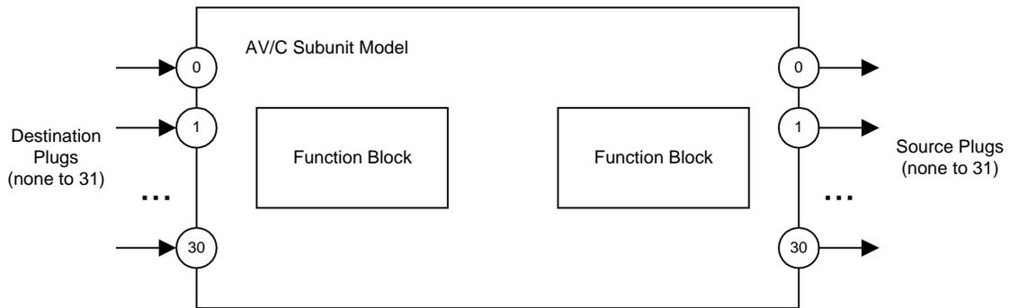
**Figure 10.2 – AV/C subunit model**
