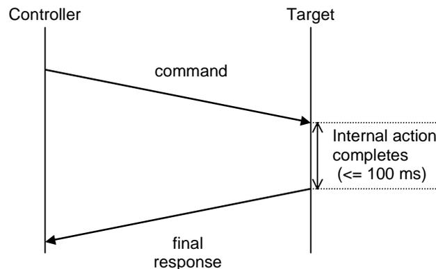
**Figure 8.1 – AV/C immediate transaction**
