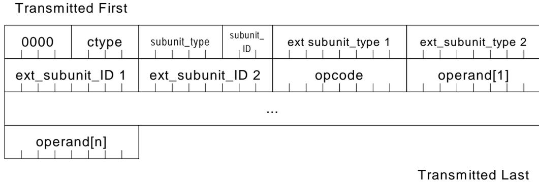
**Figure 7.3 – AV/C command frame with two extended type and ID addresses**
