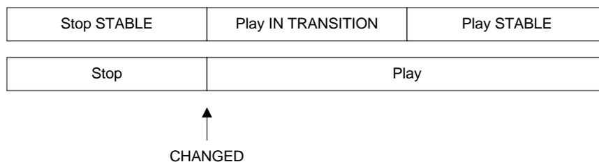
**Figure 9.5 – Timing of the CHANGED response**
