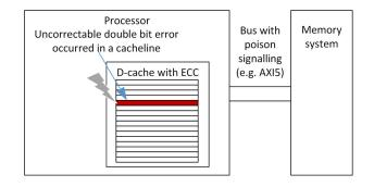
2) Later, a cache line eviction occurred, and this flushed the corrupted data. ECC error is detected at this stage and triggers the poisoning side band signal on the bus to be asserted. The poisoning state is stored in the memory system. No fault exception occurred at this stage.
