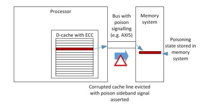
3) When the data (with poison state) is read by a processor (could be a different processor or a different bus master in the system), the poison information is passed along and triggers a fault exception at the processor.
