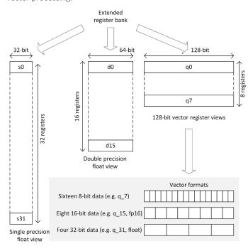
To reduce the processor's area and power, the register bank in the FPU is reused for vector processing:
