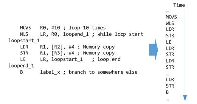
The first time the loop is executed, both WLS and LE instructions would be executed, and the loop addresses are cached inside the processor, and subsequent loop iterations do not need to execute these two instructions again. The loop counting is handled by the link register (LR/r14) and the loop exit, when the loop counter reaches zero.
