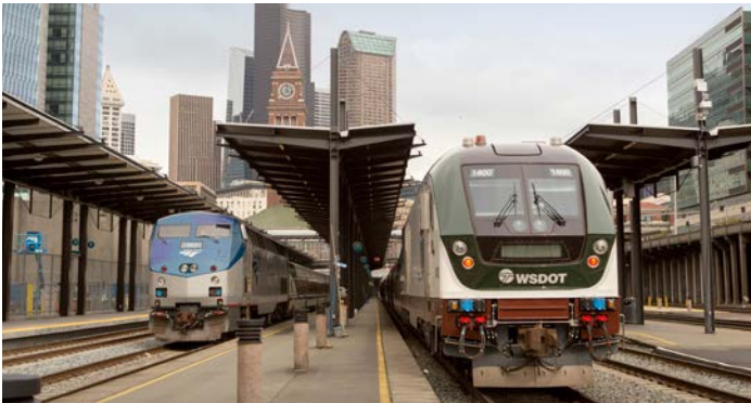
Amtrak-operated, state-owned equipment includes new diesel Charger locomotives such as the one shown at right. Owned by the Washington State Department of Transportation, it wears the Amtrak Cascades paint scheme.
