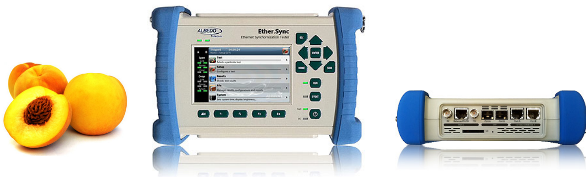
Figure 1 ALBEDO Ether.Sync is a field tester for Synchronous Ethernet equipped with all the features to install and maintain Precision Time Protocol (PTP / IEEE 1588v2), Synchronous Ethernet infrastructures, and Gigabit Ethernet supporting legacy features such as BER and RFC2544 while new test such as eSAM Y.1564.
