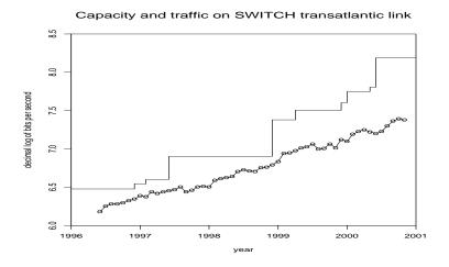
Capacity of link between the Swiss SWITCH network and the U.S., and traffic on it towards Switzerlan.
