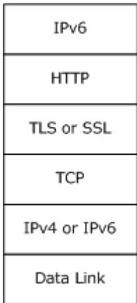
Figure 2: IP-HTTPS client protocol stack
