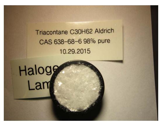
Figure 3: Triacontane loaded into IR sample cell.
