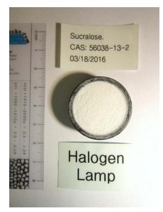
Figure 3: Sucralose loaded in IR sample cup.
