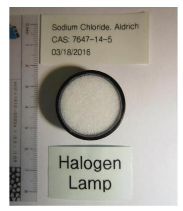
Figure 3: Sodium Chloride loaded in IR sample cup.
