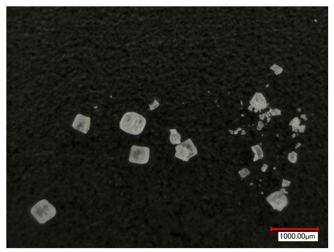
Figure 4: Photomicrograph of Sodium Chloride.
