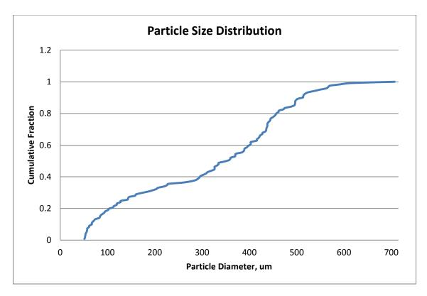
Figure 5: Particle size distribution of Sodium Chloride.
