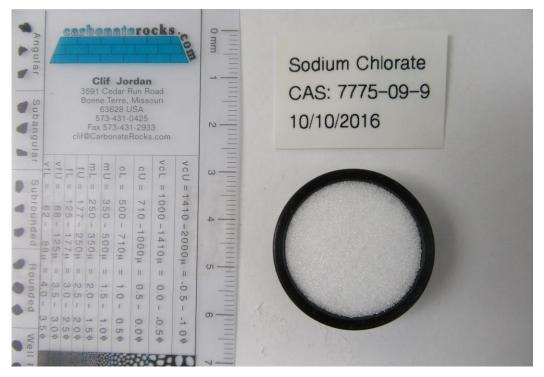
Figure 3: Sodium chlorate loaded in IR sample cup.
