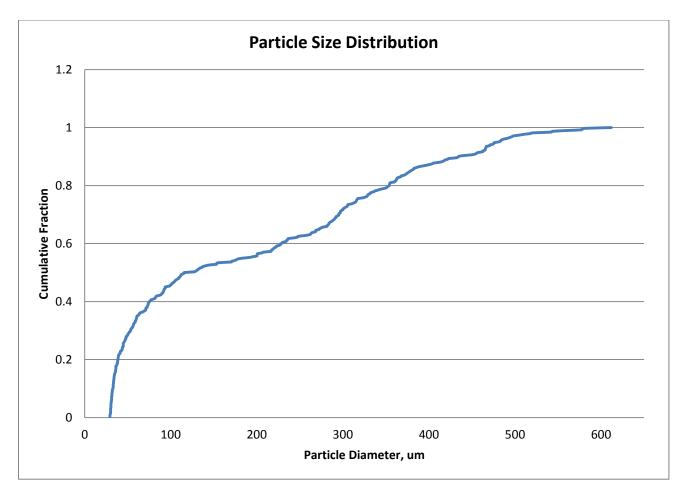
Figure 5: Particle size distribution of Sodium chlorate.
