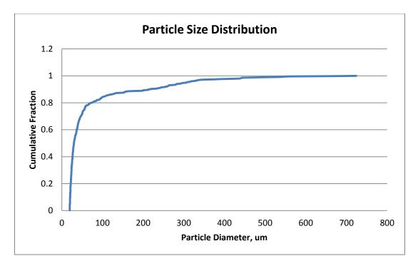
Figure 5: Particle size distribution of Sodium carbonate.
