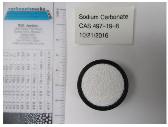
Figure 3: Sodium carbonate loaded in IR sample cup.
