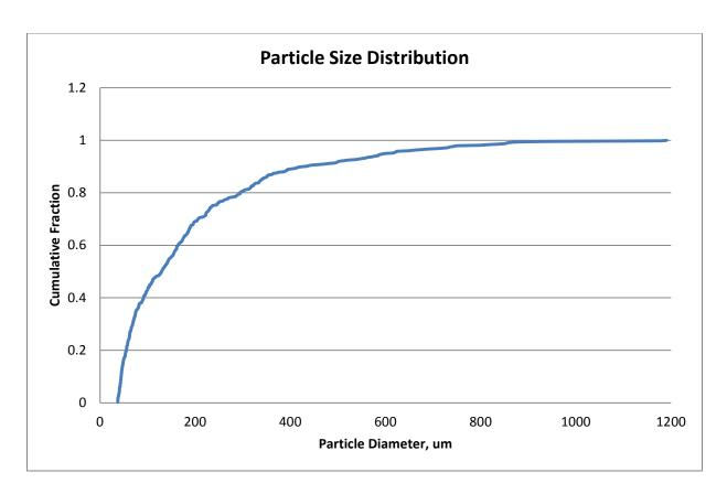
Figure 6: Particle size distribution of Potassium nitrate.
